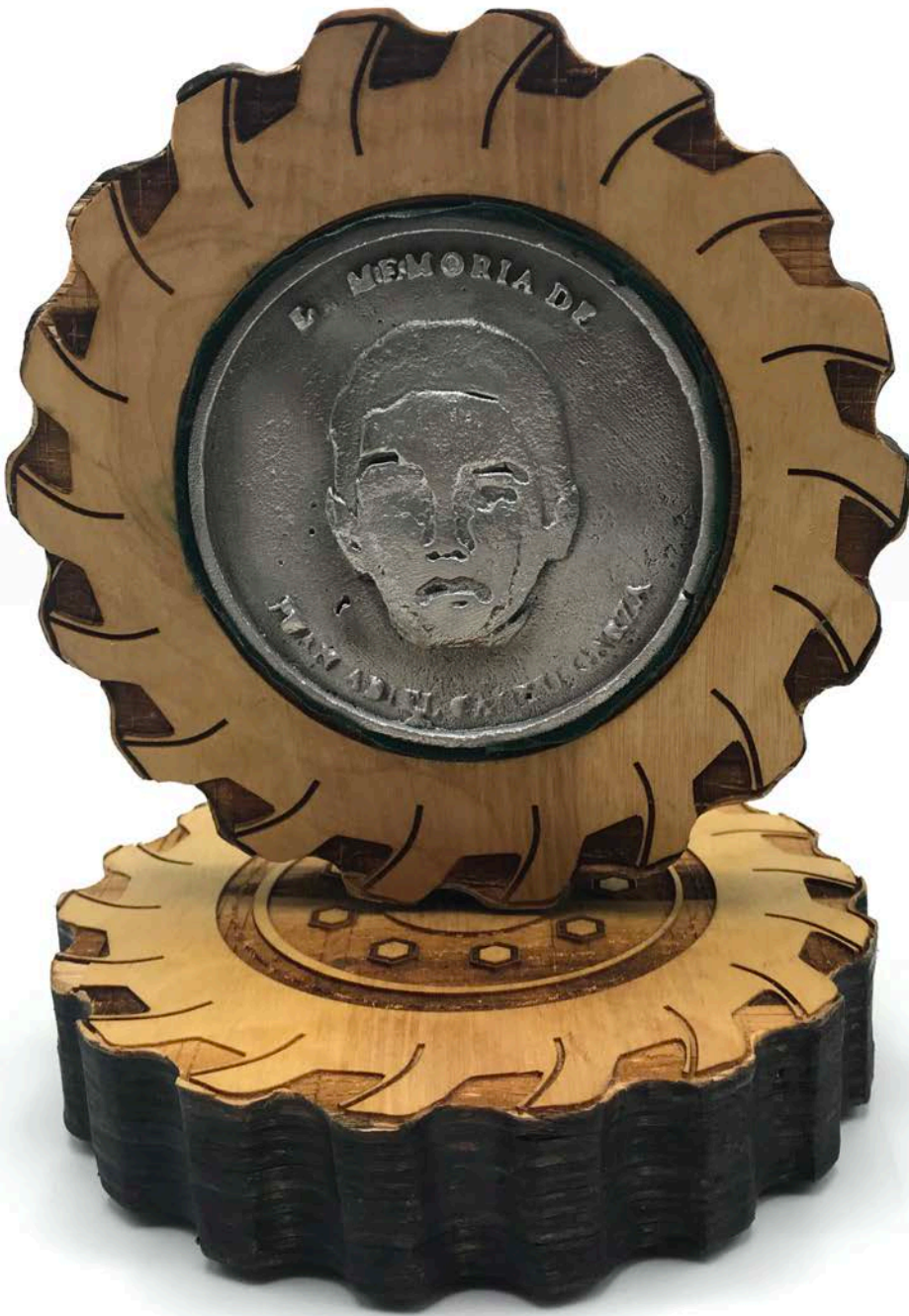
ALUMINUM CASTED COIN FROM 3D PRINT IN LASER ETCHED WOODEN DISPLAY
